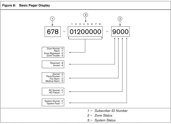
Figure 8 shows the transmission came from the control panel with an ID number of 678 and that zone 2 is in alarm. The figure also displays that zone 3 was manually isolated and the system armed.
