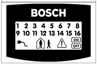
The codepad is the communications interface between you and your alarm system. Use the codepad to issue commands. The codepad offers both visual and audible indications that guide you through the general operation.
